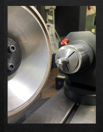
Feed across the tool at a good rpm and an even rate Stopping just before center.
