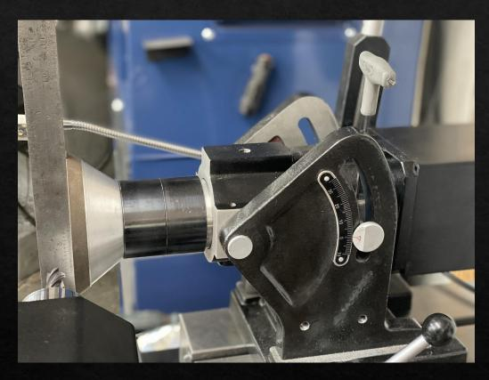
Grind the primary angle, watch your indicators. Go as close to center as you can with out taking the tips off the corners
